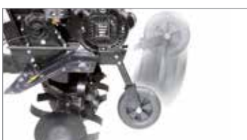
Front wheel for easy transportation of the machine. The wheel can be easily folded upward without tools to facilitate operations on the ground.
