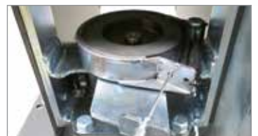
The service and parking brake engages automatically when the clutch is released, to prevent accidental hazardous movements.
