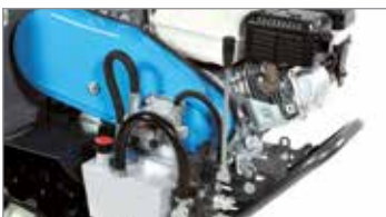
Lever-operated hydraulic tipping control valve.
