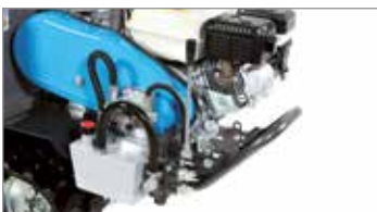
Lever-operated hydraulic tipping control valve.
