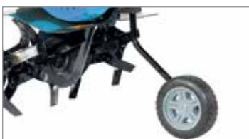
Rear wheel for easy transportation of the machine.
