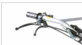
Independent brakes on each wheel supplied as standard.
